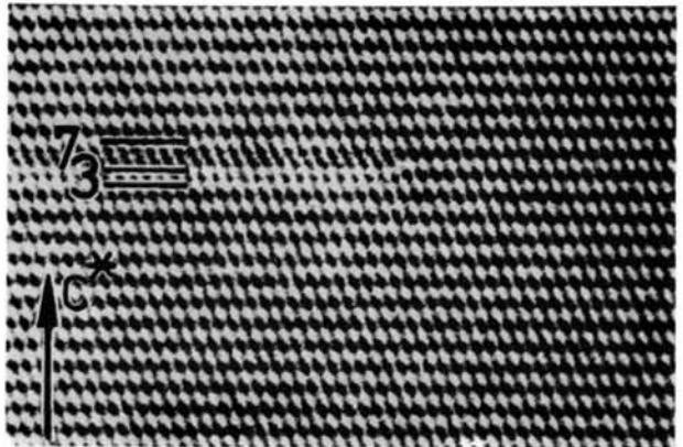
Fig. 3. Termination of periodicity faults by recombination of a pair of adjacent dreier and siebener fault units to two layers of 'right' fünfer chain units (section enlarged from Fig. 1).
